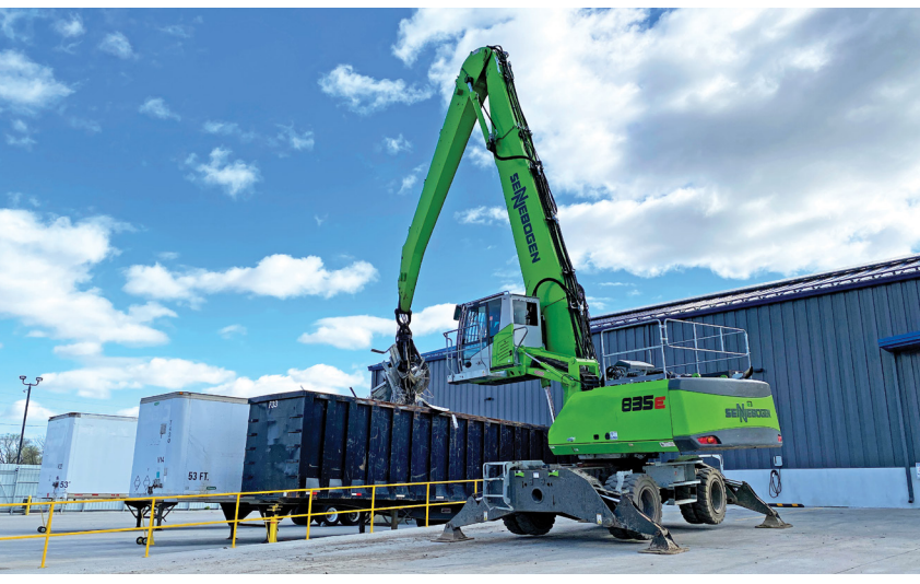
A Scrap Processors Inc. operator uses a SENNEBOGEN 835E material handler to load a shipping container with aluminum at its Des Moines, Iowa yard.
