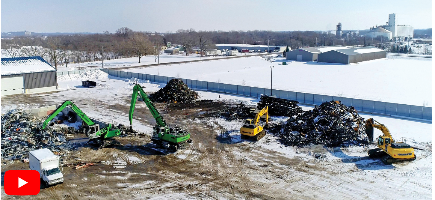
Scrap Processors Inc. (SPI) opened a new, 10-acre facility in Des Moines, Iowa in 2020. SPI uses SENNEBOGEN 825 and 835E material handlers in addition to Komatsu PC210LC and PC390LC excavators to process material at the yard.
