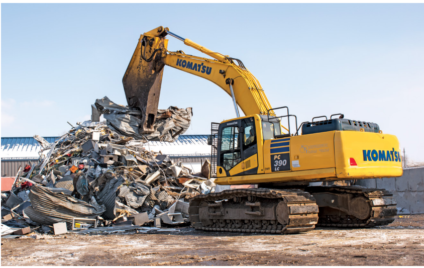
Using a Komatsu PC390LC with a Genesis GXT mobile shear attachment, a Scrap Processors Inc. operator cuts a piece of sheet metal.
