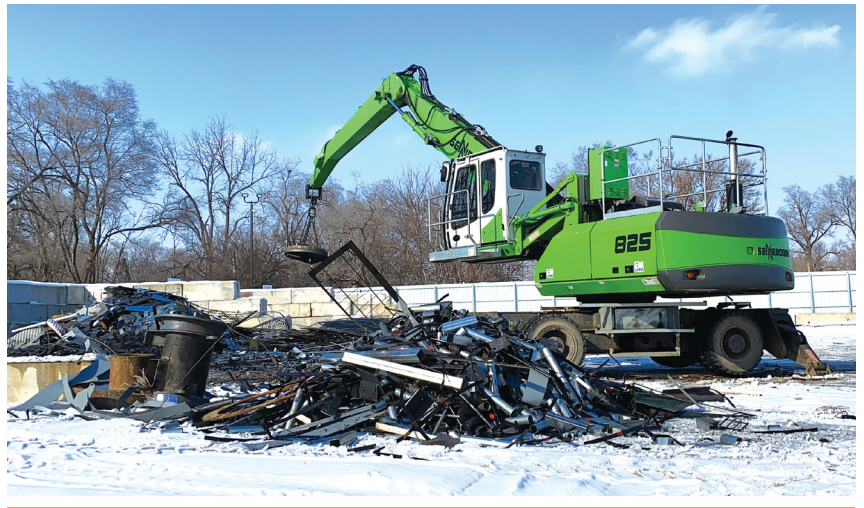
At Scrap Processors Inc.’s new Des Moines, Iowa location, an operator uses a SENNEBOGEN 825 with a magnet attachment to separate a pile of scrap metal.
